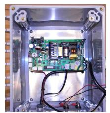
Locate fuses on back of circuit boards (indicated by the pictures) and check fuses to see if blown. Replace any blown fuses and reassemble control box in reverse of the disassembly instructions. If the fuse blows again or you still have a blank display call Clearwater Enviro Tech to obtain a RMA, DO NOT KEEP REPLACING FUSES!
