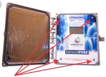
To check the fuses, open up the unit and remove the four (4) screws holding the top collar in place.
