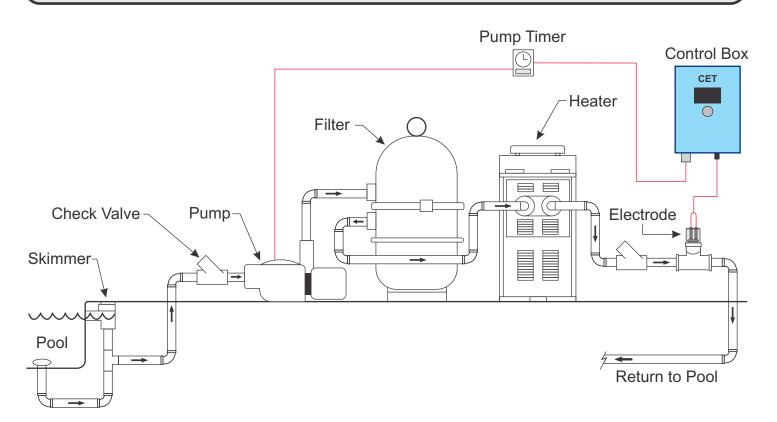
The MineralPURE unit should be installed at the pool's pump and filter area. The preferable location to mount the electrode chamber(s) is after the pools pump and filter, but it can be installed before the pools pump and filter if needed. The chamber(s) will need to be within 30 feet of the control box for an electrical connection. The control box will need to be within 11 feet of an electrical source.
