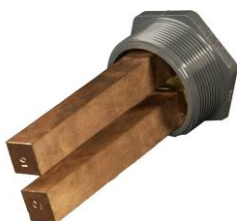
7" long 90% copper, 10% silver electrode, 3"sch 80 (CLE-20)
